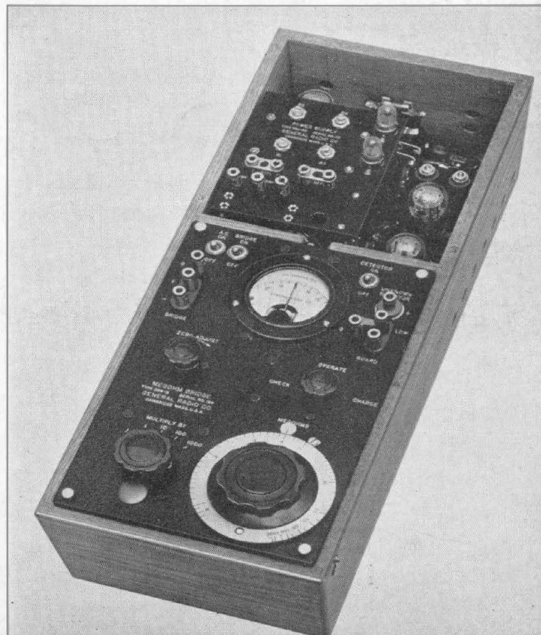
FIGURE 1. The TYPE 544-B Megohm Bridge with cover removed to show the TYPE 544-P3 Power Supply.
